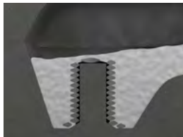
The liquid melted aluminium fills the mould and encloses the IMTEC® CO without flowing into the internal thread.
