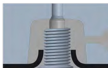
Opening the mould and demoulding
