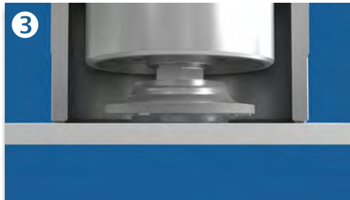
Touching the tool to the substrate
