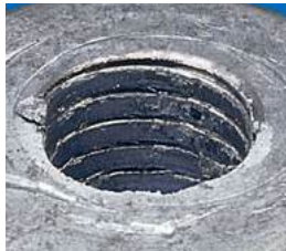
Defective thread
