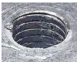
Defective thread
