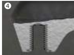
The liquid melted aluminium fills the mould and encloses the HELICOIL® Cast without flowing into the internal thread.
