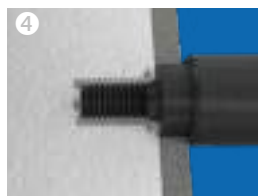
The liquid melted aluminium forced in under high pressure fills the mould and encloses the HELICOIL® Cast on the spindle core without flowing into the internal thread.
