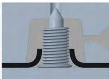
Holding pressure and cooling
