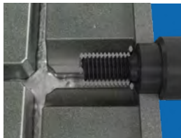
Steel mould, IMTEC® CO and automatic spindle device.
