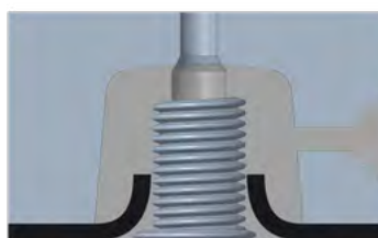
Opening the mould and demoulding
