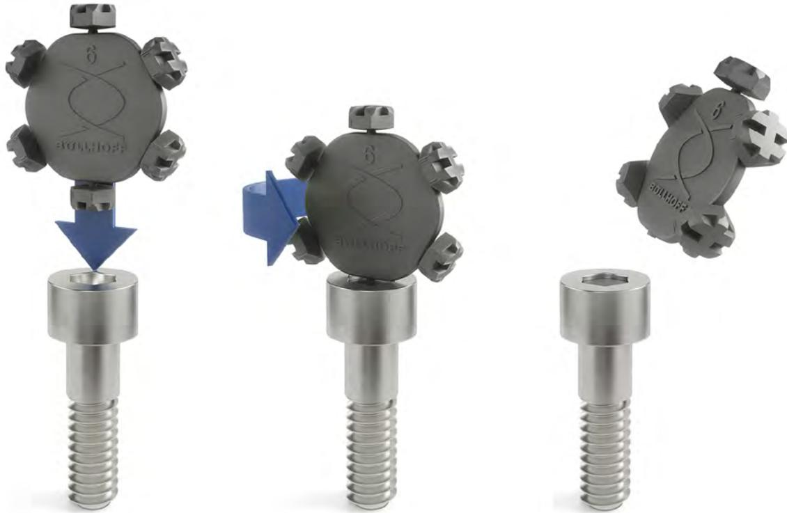
Up to six plugs can be assembled on a handling aid. This allows a simple installation without any tools. The handling aid inserts the plug into the screw recess. The handling aid is then rotated or tilted to release the plug. Once it is inserted, the PARRYPLUG® immediately provides efficient protection against unauthorised access. Quick and simple: The installation operation can be repeated without any further preparation until all of the plugs are installed.
