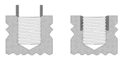
KEES are driven down into the tapped threads of the parent material during installation to securely lock the insert against rotation.
