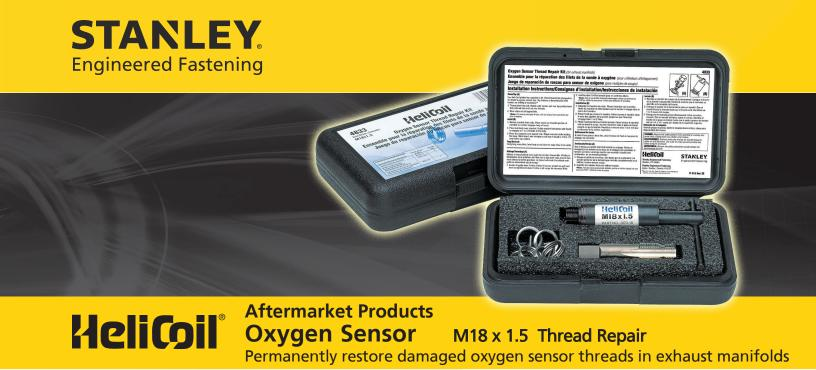
Quickly and permanently restore damaged M18 x 1.5 oxygen sensor threads in exhaust manifolds with this kit. No drilling is necessary with the piloted reamer tap, resulting in perfect alignment of the newly tapped hole.
