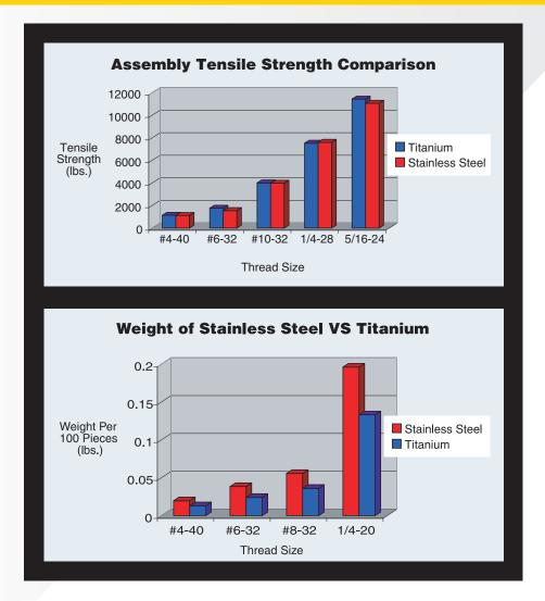
As shown in the chart above, Titanium inserts weigh significantly less than 300 series stainless steel. Weight reduction is a significant concern in Aerospace applications, where fuel consumption and efficiencies are a priority.
